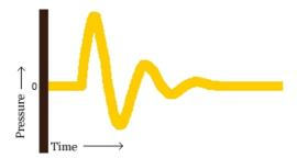
A hand clap is a short event that causes a single wave of air that quickly dies out. The image above shows the shape of the wave ("waveform") for a typical hand clap.
