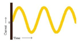
One could say that the shape of the electrical wave is *analogous to* ("similar to") the shape of the original sound wave. This is why these electrical waves that represent sound waves are called **analog waves**.
